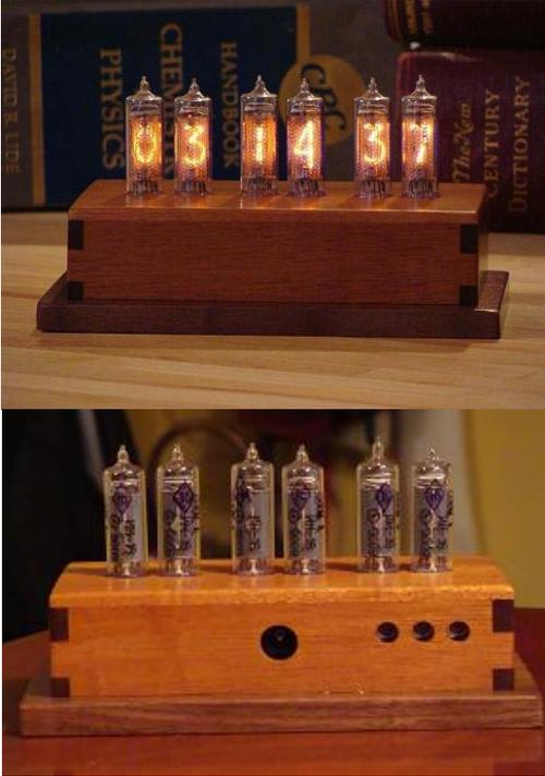
Above is the back view of the clock. The center hole is the access for the power jack. To the right are three button holes. The buttons can be accessed simply with a ballpoint pen or a pencil. Left to right, the first button is the "C" button, setting the digit cycling. The default is no cycling at all. The second button is the "M"(inute) button, setting the minutes. The last is the "H"(our) button, which sets the hours.
